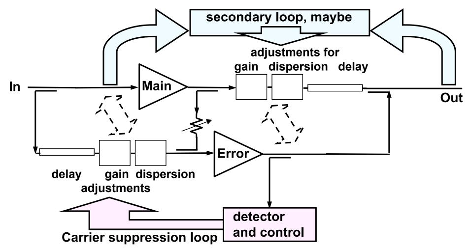
The main amplifier operates with the input signal's peak-to-average ratio. The error amplifier handles a much higher peak-to-average ratio signal, idling much of the time. If predistortion is used in the main amplifier, the error amplifier has an even more peaky signal to amplify, nearly impulses. Therefore, the frequency response of the error amplifier must be super.
