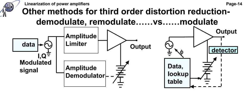
Very efficient approach, limited by the load impedance variation and voltage breakdown
