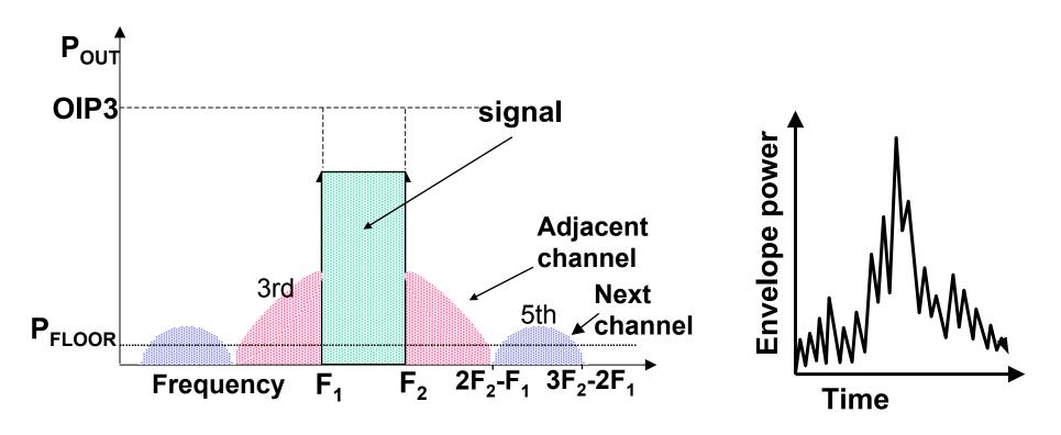
The n signals making up the channel can add up at times to a peak power level as large as n times the total average power. Although this is only occasional, the limiting that occurs generates higher order distortion. Thus, the OIP3 performance can be overshadowed by the peak power performance of the amplifier. The slope of the adjacent channel interference is due to the probability of the third order IM products falling at that frequency.
