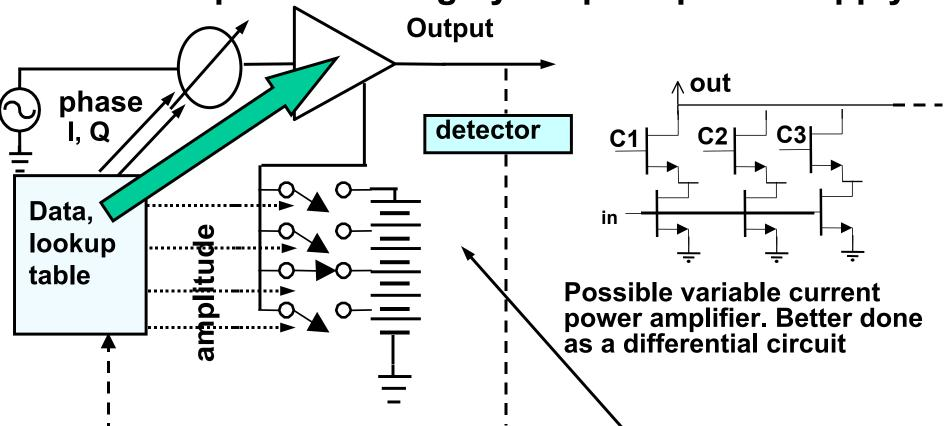
Just before the moment a larger supply voltage is needed for linearity, the supply voltage switches. Note that the dc-dc converter does not need to follow the modulation.
