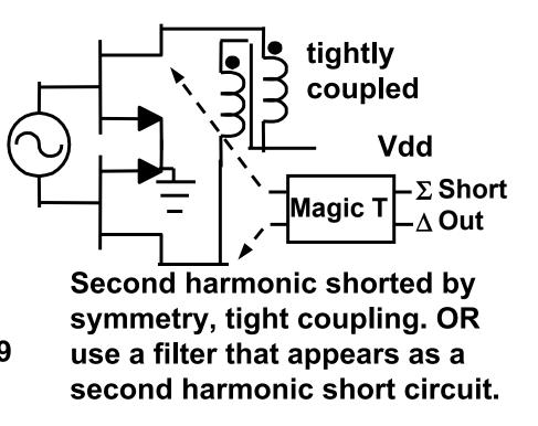
Note the VPO shift with VDS, this effectively adds in the output voltage. It is important to eliminate second harmonic at the FET output. For wideband (> octave), a symmetric short is imperative!
